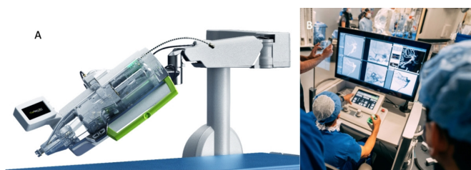
Figure 2 CorPath GRX Robotic System. (A) Robotic arm with advanced cassette. (B) The set-up of the procedure. The primary neurointerventionalist was located in the corner of the angiography room in a radiation-shielded workstation. At bedside, the team consisted of the specialised robotic technologist and two neurointerventionalists who load the devices and control the perfused lines and hubs.
