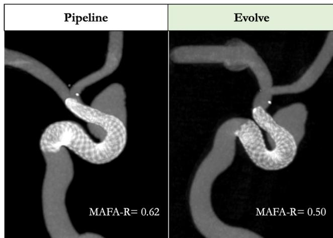
**Figure 1** Representative views of 3D Vaso-CT imaging demonstrating wall opposition after angioplasty of both a Pipeline Flex (4.25×25 mm) and a Surpass Evolve (4.25×25 mm) stent, sequentially placed in the same patient-specific silicone aneurysm model. MAFA-R, mean aneurysm flow amplitude ratio.
